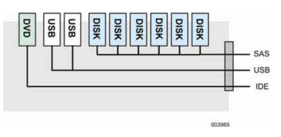
Figure 2-12 Peripherals on the Drive Tray
